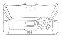
Please use a pry tool to conceal the power line under the roof upholstery and seal the rubber ring along the A-pillar.
