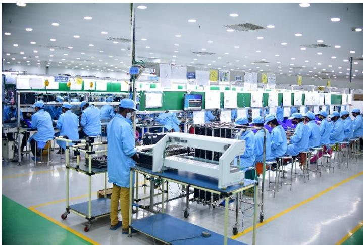
The CP PLUS manufacturing facility Kadappa in the state of Andhra Pradesh has been integrated with the world's latest Fuji made state-of-the-art technology SMT Lines and semi-Robotic Assembly & packaging Lines. All production area has been designed with ESD flooring, dust-free and air-conditioned environment to achieve world's best quality of products.
